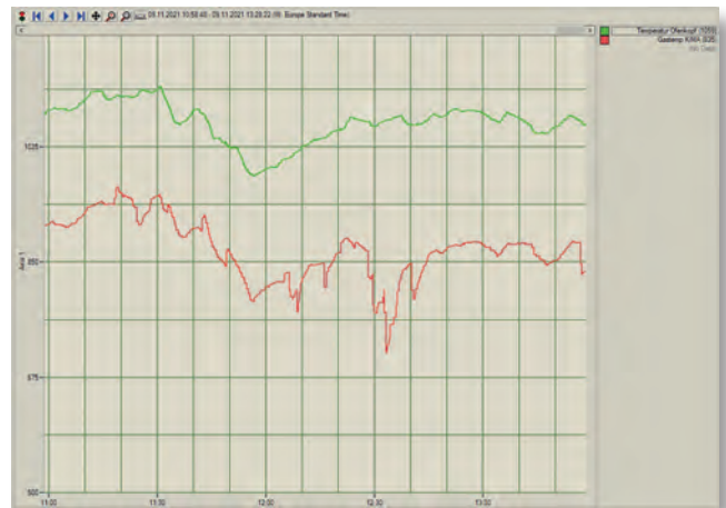
Figure 14: Average temperature – fast, short drop due to air blaster
