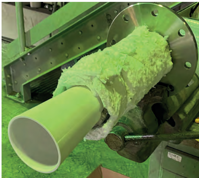
Figure 7: Acoustic horn, consisting of ceramic for up to 1600 °C
