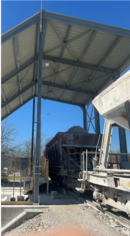
Wagon unloading station for limestone with downstream conveying
