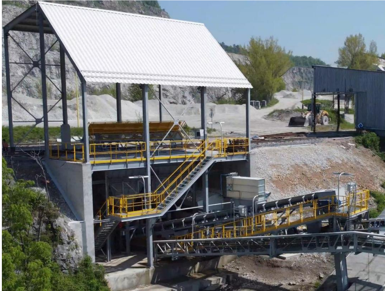
Wagon unloading station for limestone with downstream conveying
