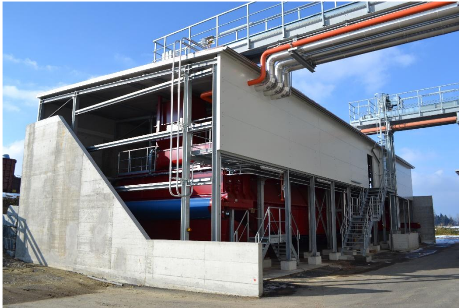
Belt Dryer in Ruyères, CH , 6.7 t/h – 130 m 2 drying of Sawmill (Wood pellets)
