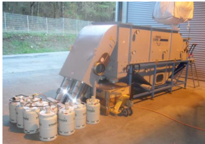
Belt Dryer continuous test plant – 2 m 2
