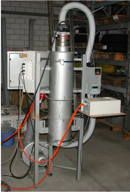
Static Test Dryer (product samples 5 kg batch)
