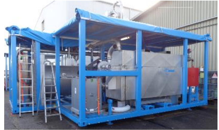
ecoDry – Evap ca. 100 kg/h test plant
